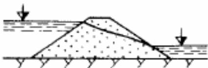
Figure 2.1 Homogeneous embankment dam [*Goldin and Rasskazov*, 1992]
