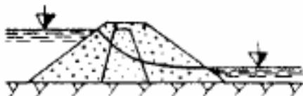
Figure 2.2 Zoned embankment dam with thin central core [Goldin and Rasskazov, 1992]
